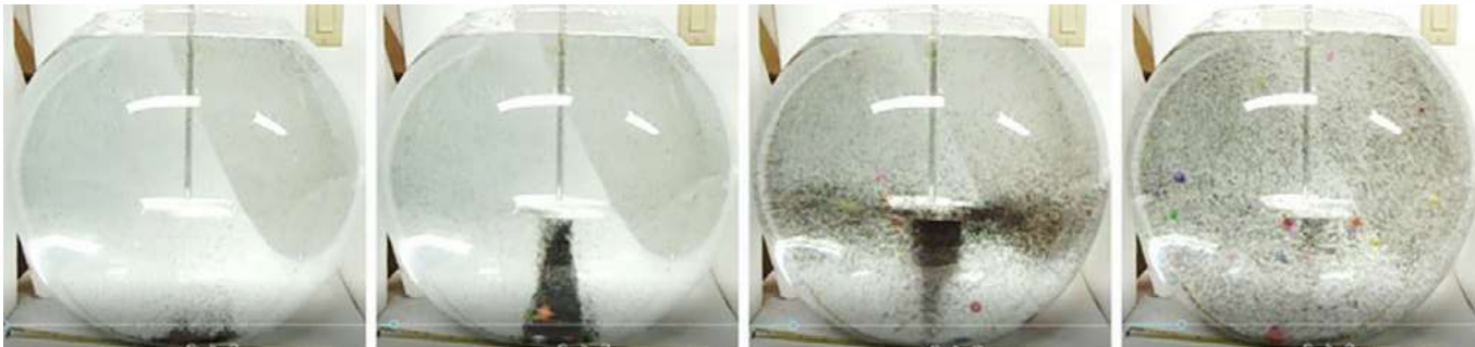
Figure 1. The high performance centrifugal dispersing impeller (HPCDI) suspends solids with a tornado like force.
