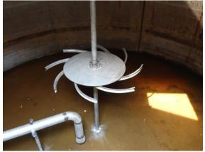
**Top:** HPCDI lifts water toward the impeller with a tornado-like swirling movement. At the tank bottom, this swirling movement sweeps the solids to the centre where they are suspended.
